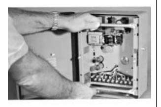
2. Fireye 25SU5 controls may be wired and operated in a variety of methods. The circuit diagram on page 3 illustrates the interconnection between the 25SU5 and 70D40-41 control. It shows the recommended method of connecting the supply, limit switch, and momentary start switch, as well as the two SPDT relay circuits whose function is the same for both 25SU5 and 70D40-41 controls. All wiring must have 600 volt insulation.
