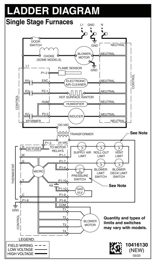
Figure 37. Emerson Ladder Diagram
