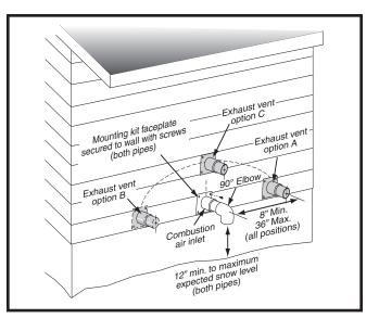
Figure 7. Inlet & Exhaust Pipe Clearances
