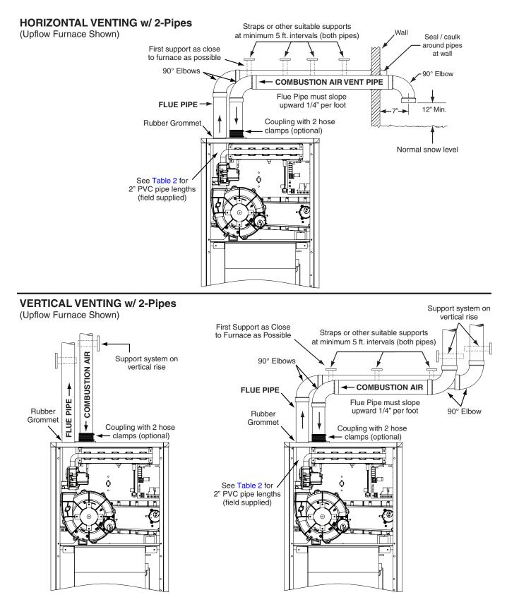
Figure 38. Horizontal & Vertical Venting
