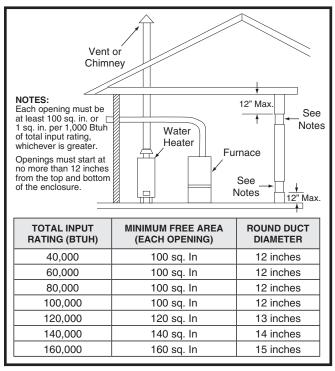
Figure 2. Combustion Air Drawn from Inside
