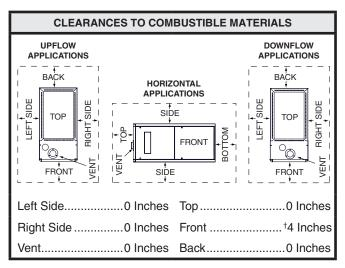
$\ensuremath{+}\xspace$  Allow 24 in. minimum clearance for servicing. Recommended clearance is 36 in.
