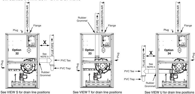
Figure 46. Venting Options for Downflow Installations (\*SM Series)
