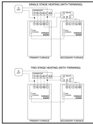
Figure 30. Emerson Single & Two Stage Twinning
