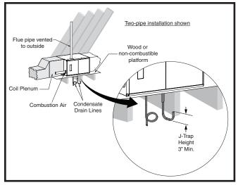
Figure 11. \*SC & \*SD Horizontal installation on a Platform
