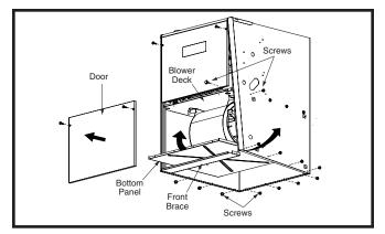
Figure 23. Alternate Removal Method
