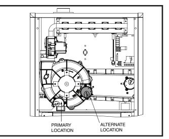
Figure 17. Alternate Pressure Switch Location
