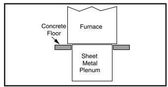
Figure 13. Furnace on a Concrete Slab
