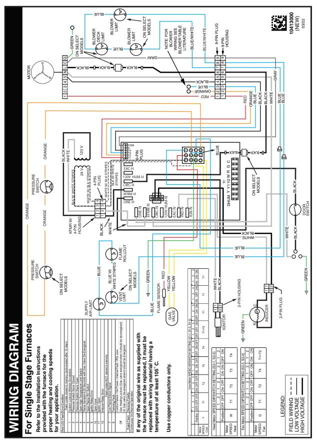
Figure 35. Emerson Wiring Diagram
