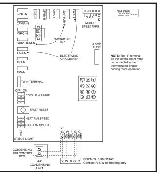
Figure 28. Emerson Low Voltage Field, Fourwire Heating/Cooling Applications
