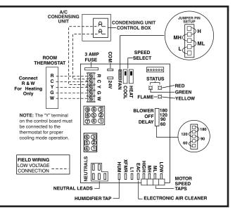
Figure 27. Nordyne/UTEC Low Voltage Field, Fourwire Heating/Cooling Applications
