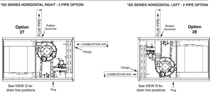
Figure 45. Venting Options for Horizontal Installations (\*SD Series)
