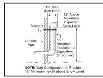
Figure 9. Alternate Horizontal Vent Installation
