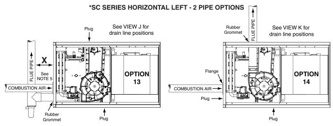
Figure 41. Venting Options for 2-Pipe Horizontal Installations (\*SC Series)
