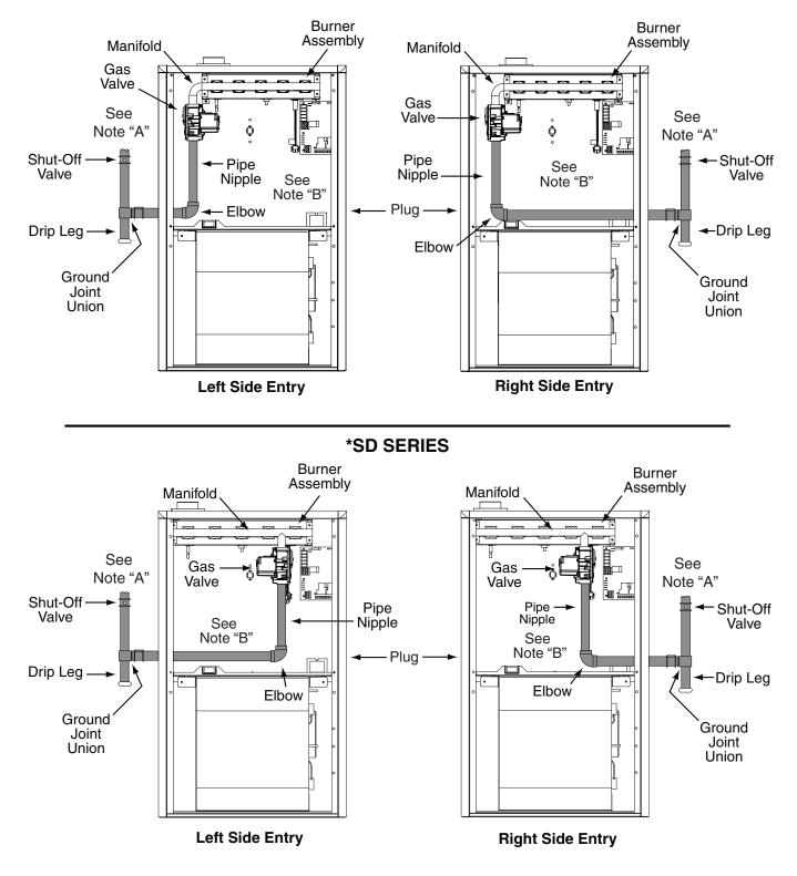
NOTE A: Consult local codes for Shut-Off Valve location requirements NOTE B: Inducer assembly omitted for clarity of pipe installatio
