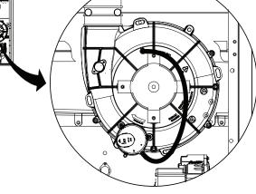
Figure 16. Pressure Switch Tubing for Downflow Furnaces Models \*SL072, \*SM054, \*SM072, & \*SM090
