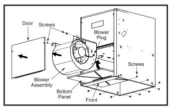
Figure 22. Bottom Panel Removal
