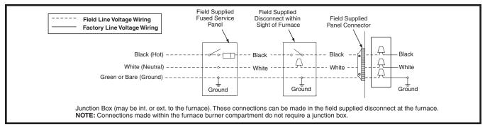
Figure 26. Line Voltage Field Wiring
