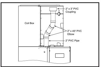
Figure 21. Optional PVC Pipe Installation
