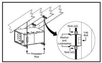
Figure 12. \*SC & \*SD Horizontally Suspended in an Attic
