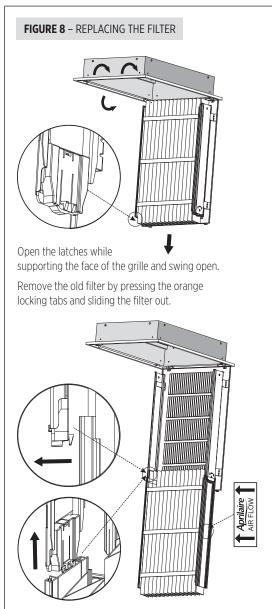
Align new filter in both rails and slide into place with "Air Flow" pointing away from the grille. The end cap of the filter should be placed on top of the orange locking tab to depress it before sliding into the rail.
