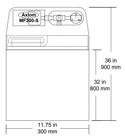
Depth - 11.75 in 300 mm Clearances – Right Side - 12 in 305 mm Weight When Full 157 lbs/72 kg. Discharge 1/2" FPT
