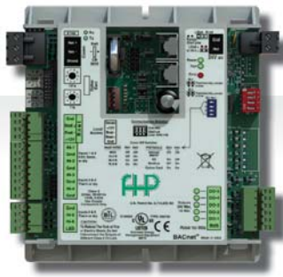
DDC Control Board
