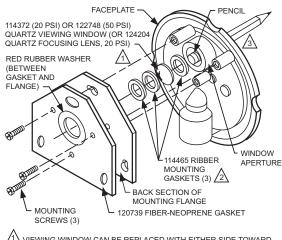
1 VIEWING WINDOW CAN BE REPLACED WITH EITHER SIDE TOWARD THE FLAME.
