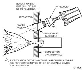
Fig. 5. Typical mounting of C7961.
