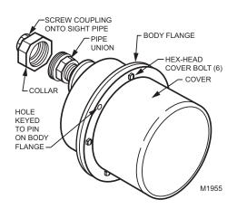
Fig. 9. Mounting a C7961F Detector.
