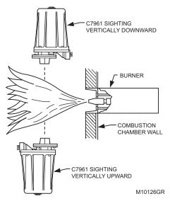
Fig. 6. Vertical mounting of C7961E.
