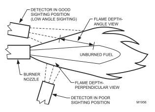
Fig. 3. Detector sighting angle.
