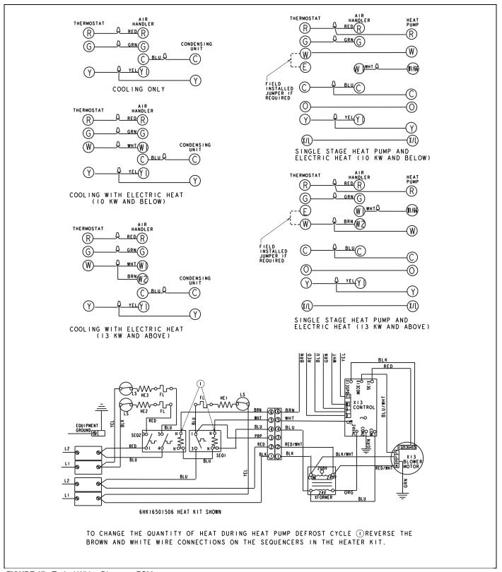
FIGURE 17: Typical Wiring Diagram - ECM
