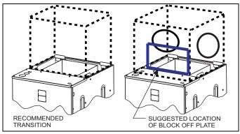
FIGURE 9: Ductwork Transition
