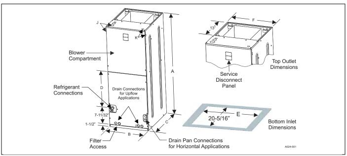
FIGURE 2: Dimensions & Duct Connection Dimensions
