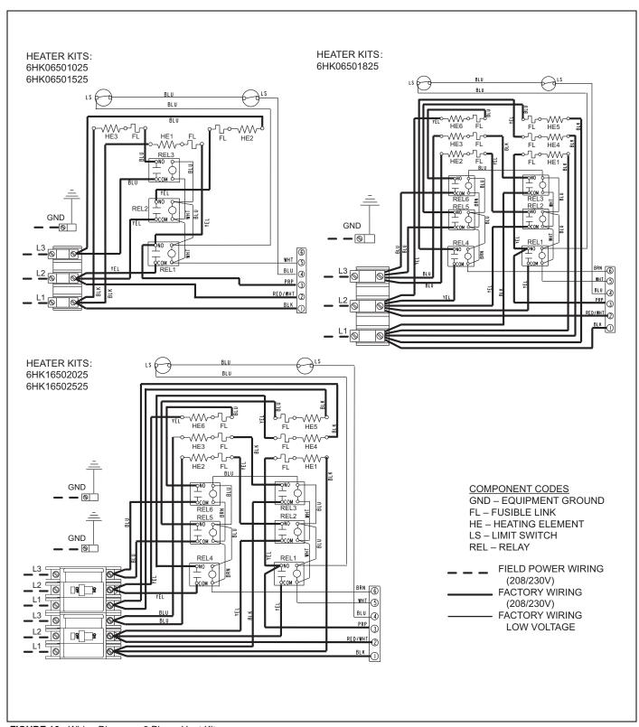
FIGURE 16: Wiring Diagram - 3 Phase Heat Kits
