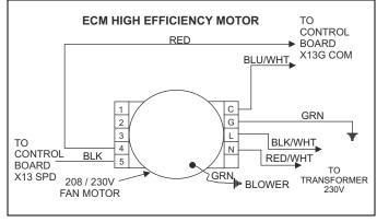
FIGURE 14: Blower Speed Connections
