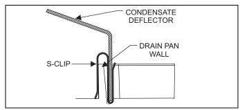
FIGURE 6: S-Clip Installation
