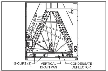
FIGURE 4: Condensate Deflector on Vertical Drain Pan
