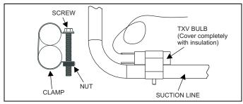
FIGURE 11: Proper Bulb Location
