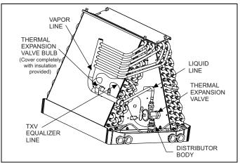
FIGURE 10: Thermal Expansion Valve (TXV)
