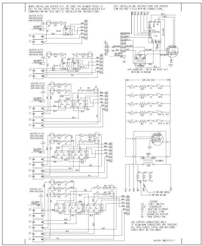
FIGURE 15: Wiring Diagram - ECM - Single Phase Heat Kits
