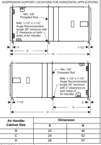
FIGURE 7: Horizontal Suspension
