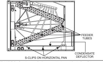
FIGURE 5: Condensate Deflector on Horizontal Drain Pan Edge
