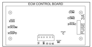
FIGURE 12: Blower Delay Control Board
