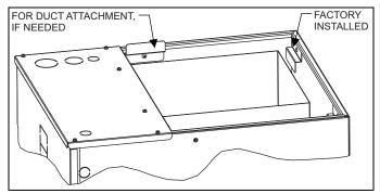
FIGURE 8: Duct Attachment
