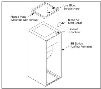
FIGURE 11: Blower Bracket and Duct Flange Attachment
