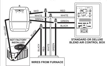
Four-conductor wire is required for thermostat connection. Attach the 4 low voltage wires extending from the control box as follows:
