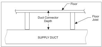
FIGURE 3: Duct Connector Depth (7990 Series)
