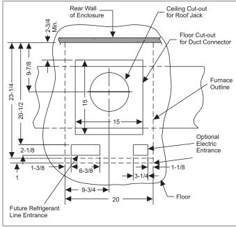
FIGURE 5: Recommended Floor Cut-out (7990 Series)
