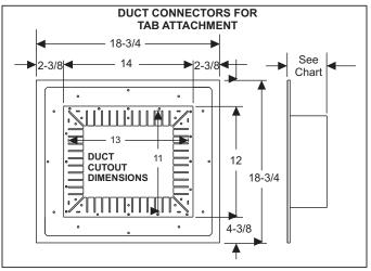
FIGURE 4: Duct Connector Dimensions (7990 Series)
