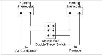
FIGURE 14: Thermostat Wiring
