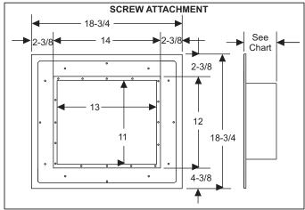
FIGURE 4: Duct Connector Dimensions (7990 Series)
