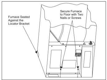
FIGURE 9: Installation of Furnace
