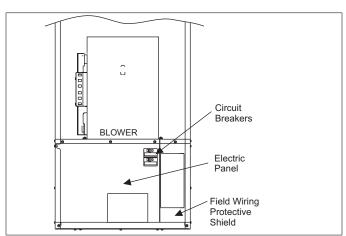
FIGURE 13: Field Wiring Shield
