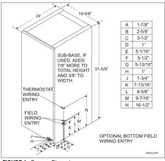
FIGURE 1: Furnace Dimensions
