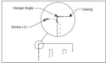
FIGURE 10: Hanger Angle Attachment
