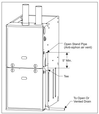
FIGURE 20: Typical. Condensate Drain, Vertical Installation
