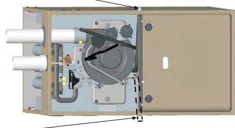
For 100 & 120 input furnaces, the condensate drain is plumbed toward the left casing outlet from the factory.
