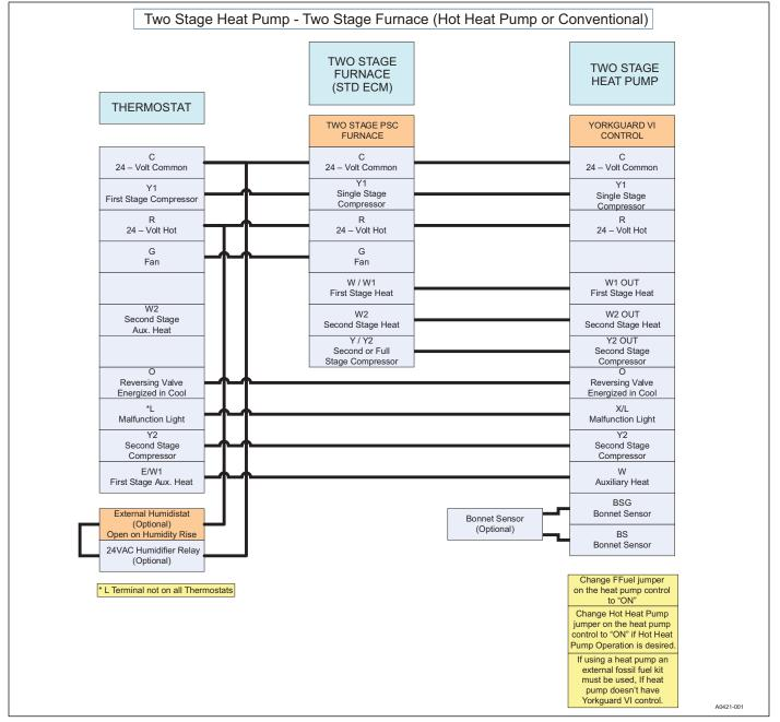
FIGURE 19: Thermostat Chart - Two Stage HP with Two Stage Standard ECM Furnace
