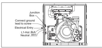
FIGURE 17: Electrical Wiring
