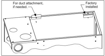
FIGURE 1: Duct Attachment
