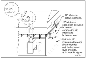
FIGURE 29: Termination Configuration - 2 Pipe Basement
