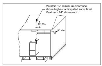
FIGURE 27: Termination Configuration - 1 Pipe
