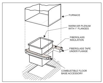
FIGURE 8: Combustible Floor Base Accessory
