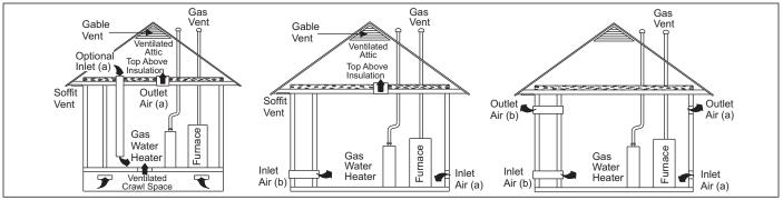
FIGURE 35: Ambient Combustion Air
