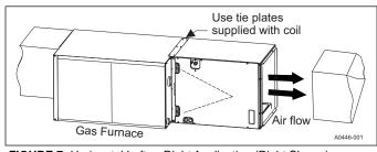
FIGURE 7: Horizontal Left or Right Application (Right Shown)
