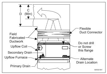
FIGURE 6: PC Series Upflow Coil Installation
