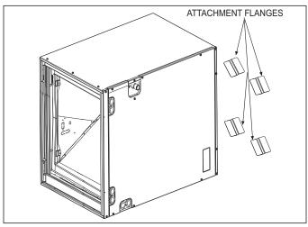
FIGURE 3: Coil Cabinet Attachment Flanges
