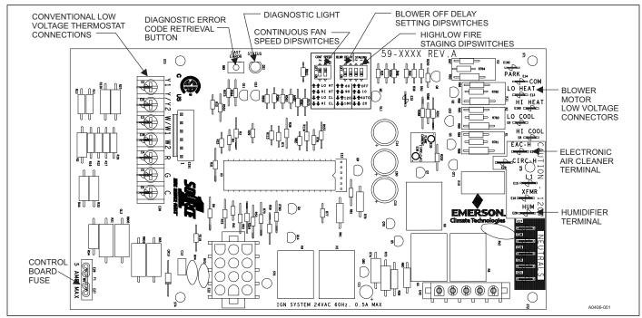
FIGURE 40: Furnace Control Board
