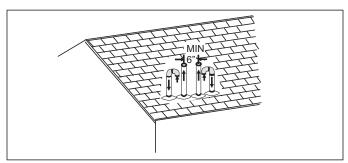
FIGURE 31: Double Vertical Combustion Air Intake and Vent Termination
