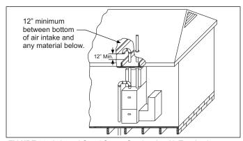
FIGURE 36: Attic and Crawl Space Combustion Air Termination
