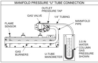
FIGURE 38: Reading Gas Pressure
