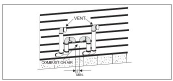
FIGURE 30: Double Horizontal Combustion Air Intake and Vent Termination
