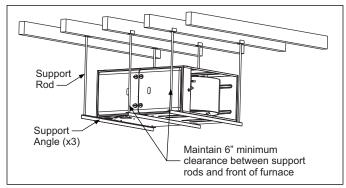
FIGURE 11: Typical Suspended Furnace / Crawl Space Installation
