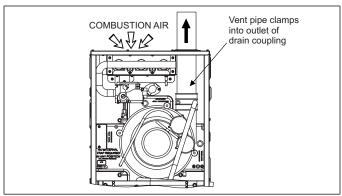
FIGURE 34: Combustion Airflow Path Through The Furnace Casing
