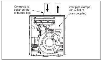
FIGURE 33: Direct Vent Air Intake Connection and Vent Connection
