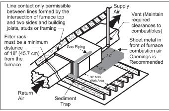
FIGURE 10: Typical Attic Installation
