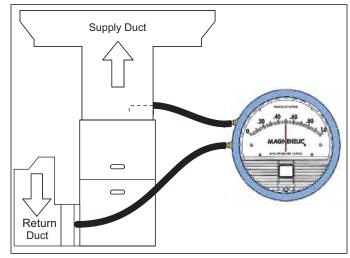
FIGURE 39: Measuring External Duct Static
