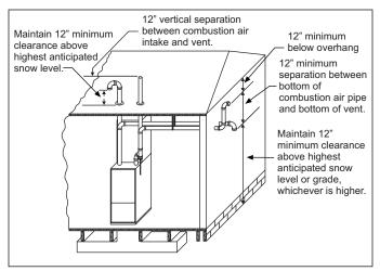
FIGURE 28: Termination Configuration - 2 Pipe
