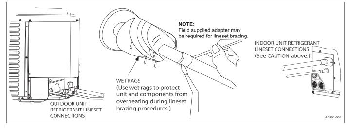
\*For unit lineset brazing precautions, refer to the Installation Manual included with the unit.
