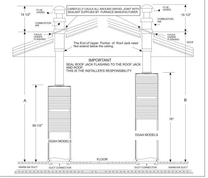
FIGURE 21: Standard Roof Jack
