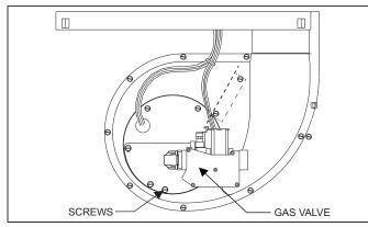
FIGURE 15: Burner Assembly
