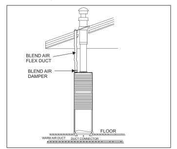
FIGURE 12: Floor Installation
