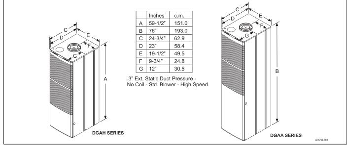
FIGURE 1: Furnace Dimensions
