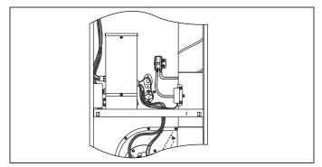
FIGURE 28: Pressure Switch Tubing Routing
