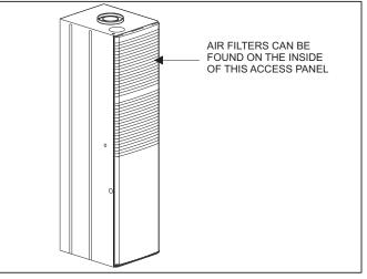
FIGURE 13: Furnace Air Filters
