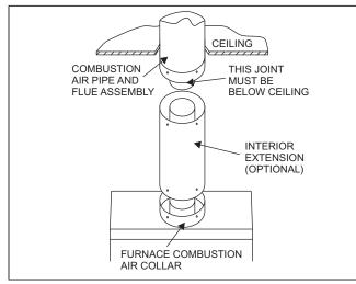
FIGURE 25: Roof Jack Assembly
