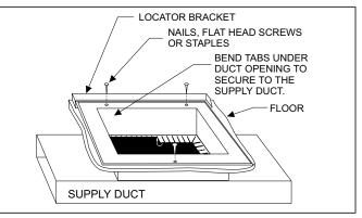
FIGURE 10: Duct Connector Tab Attachment
