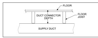
FIGURE 8: Duct Connector Depth
