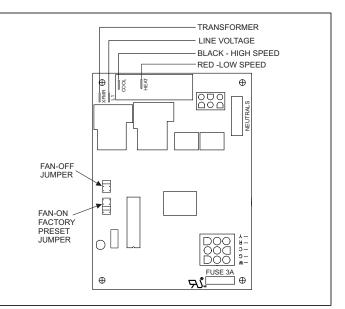
FIGURE 31: Furnace Control Board
