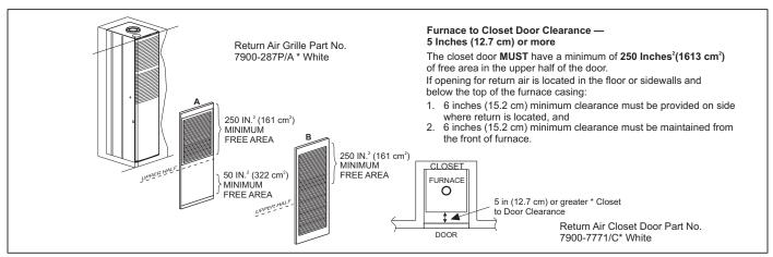
FIGURE 3: Closet To Door Clearance - 5" or Greater
