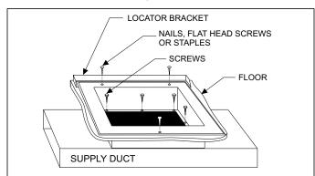
FIGURE 9: Duct Connector Screw Attachment
