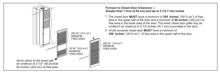
FIGURE 4: Furnace To Closet Door Clearance - 1" To 5"
