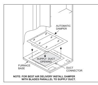
FIGURE 11: Anti-Backflow Damper
