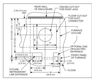
FIGURE 7: Recommended Floor Cut-out
