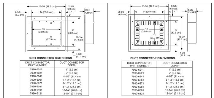
FIGURE 6: Duct Connector Dimensions
