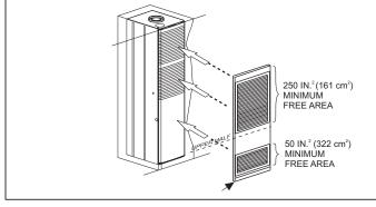
Furnace to Closet Door Clearance — Less than 1 Inch (2.54 cm)
