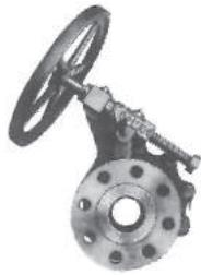
Line pressure and heavy spring hold disc firmly against the body seat, sealing off the flow. When operated, the disc slides across the body seat pushing harmful boiler scale away, and wiping clean the precision lapped surfaces.
