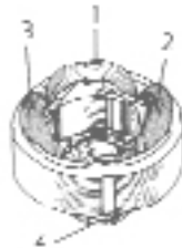
Figure 2 Shaded-Pole Motor Coils
