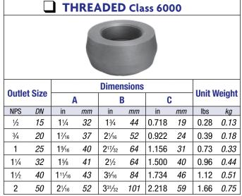
Each outlet size listed is available to fit any run curvature. Threaded ends are in accordance with ANSI/ASME B1.20.1. Design per MSS-SP-97.
