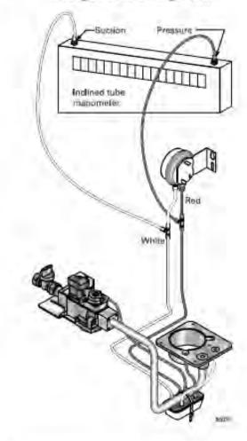
If manometer reading is at least 1.0" w<sub>i</sub>c<sub>n</sub> but there is not 24 VAC between both air pressure switch terminals and ground, replace air pressure switch.
