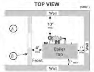
A Area adjacent to access door must be accessible and must allow for removal of the GV90+boiler for service.
