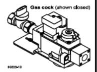
Rotate gas cock counterclockwise to open. When open, rotate clockwise to close (See below.)
