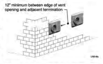
Figure 45 Hole preparation in wall — Weil-McLain vent/air plate (use template provided)
