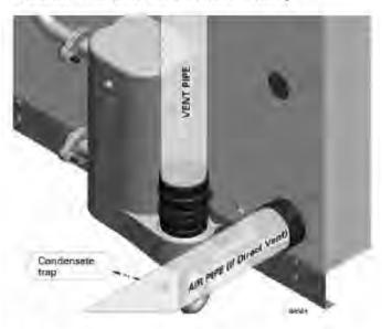
If the vent piping cannot be moved, then cut the flue pipe carefully so a coupling can be inserted later, or remove a section of vent pipe if using stainless vent pipe.
