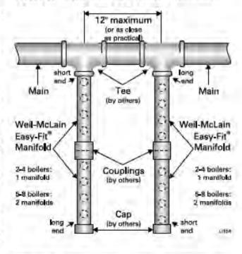
Figure 31 Double-sided EZ-Fit Header connection
