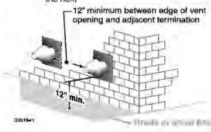
Figure 52 Installing and supporting the concentric sidewall vent assembly
