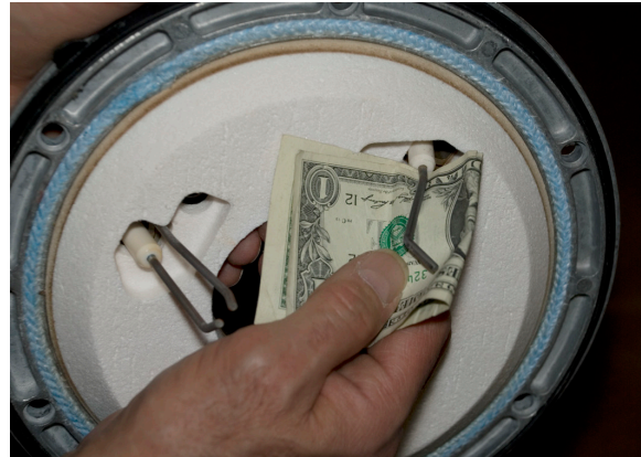
Fig. C5-10 - Correct way to clean the flame sensor
