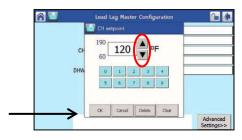
3. After adjusting the DHW set point, press "OK'.
