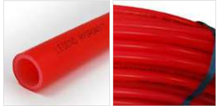
The externally extruded EVOH oxygen barrier reduces oxygen molecule permeation into the water. Compliant with standard DIN4756 (< 0.1 grams/m²/day).
