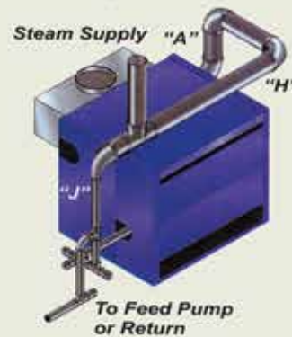
Recommended Minimum Pipe Sizes For Dual Risers
