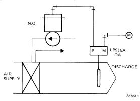
Fig. 1. Typical LP916A duct-mounted heating application.
