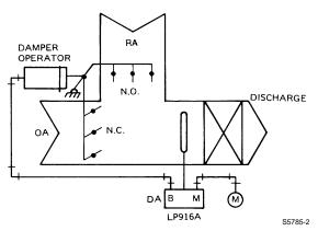
Fig. 2. Typical LP916A mixed air application.
