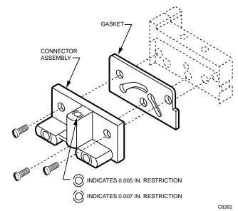
Fig. 8. Repair kit 14003113-002 (0.007 in. restriction included in kit).
