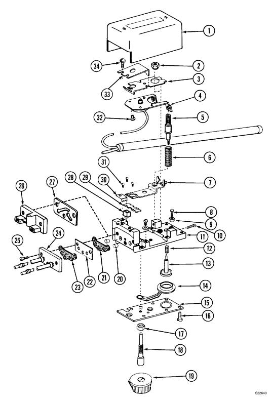
Fig. 10. LP916B Exploded view.
