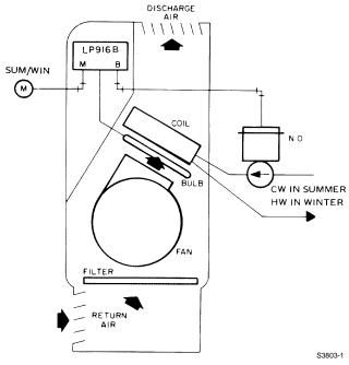
Fig. 3. Typical LP916B fan coil application, heating/ cooling with seasonal changeover.
