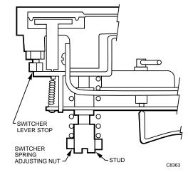
Fig. 6. LP916B Automatic switchover mechanism.
