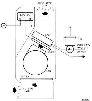
Fig. 4. Typical LP916C fan coil application, cooling only.
