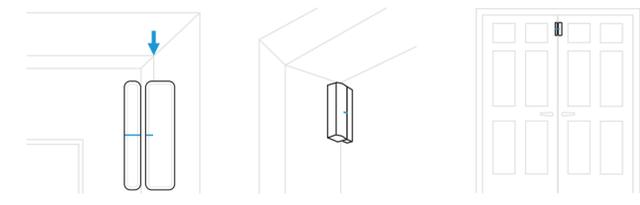
The Large Half can hang off the edge of the frame, if the space between the frame and door is greater than 1/4 inch.
