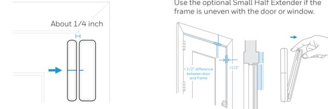
Use the optional Small Half Extender if the frame is uneven with the door or window.
