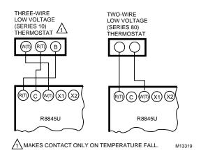
Fig. 8. R8845U thermostat connections.
