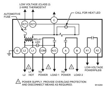
Fig. 2. R8845U Internal schematic and typical hookup.
