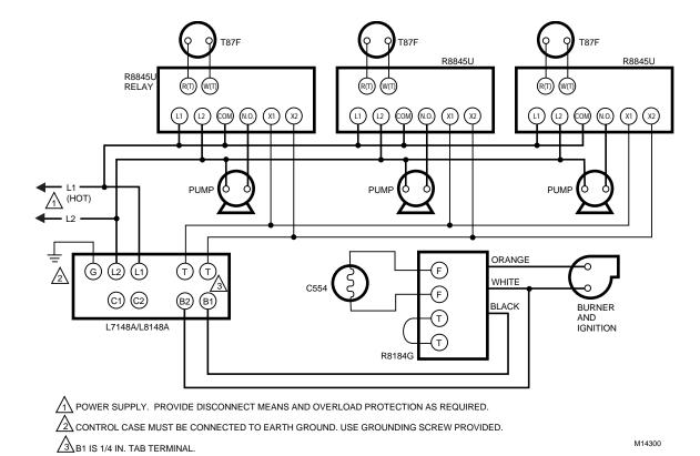
Fig. 5. R8845U hookup for L7148A/L8148A in an oil-fired, tankless hot water, zoned, pump system.
