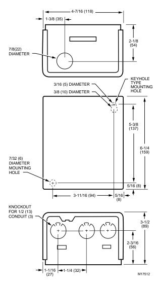
Fig. 1. R8845U dimensions in in. (mm).
