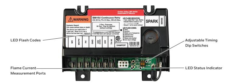
Suitable for use with or without vent dampers the S8610U provides the ignition sequence, flame monitoring and 100 percent safety shutoff for intermittent pilot central furnaces and heating appliances. Enhancements that improve the performance and simplify troubleshooting highlight the latest release of the Universal control.
