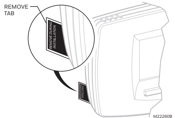
Fig. 24. Remove tab labeled REMOVE from thermostat back.
