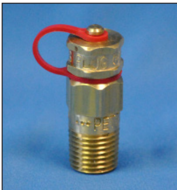
Product: #100BSP Core: Neoprene Thread: 1/4" BSP Length: 1 1/2"
