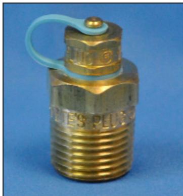
Product: #900 Core: Neoprene Thread: 1/4" NPT Length: 1 1/4"
