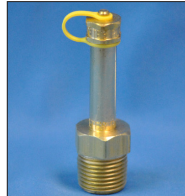
Product: #710XL Core: Nordel Thread: 1/2" NPT Length: 3"
