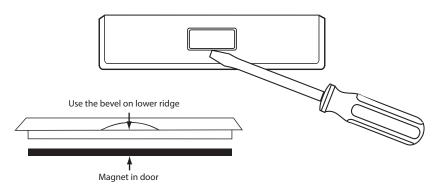
Gently slide a screwdriver into the bottom edge of the badge. Gently turn the screwdriver counter clockwise. The badge is held on by a magnet in the well of the battery door. The badge should pry off easily. DO NOT USE FORCE.
