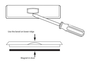
Gently slide a screwdriver into the bottom edge of the badge. Gently turn the screwdriver counter clockwise. The badge is held on by a magnet in the well of the battery door. The badge should pry off easily. **DO NOT USE FORCE.**
