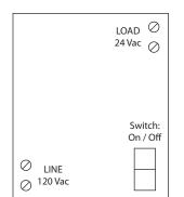
**PSMN40A** 2.75" Track Mount 40 VA Power Supply, 120 Vac to 24 Vac
