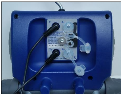
Figure 7: Connecting the Temp Probes
