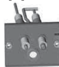
Figure 76 Correct orientation of ignition electrode / flame sense rod sight glass in down position.
