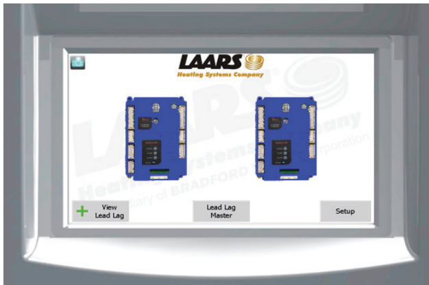
Figure 24. Touch Screen, shown with the ‘home’ screen of a SINGLE boiler configuration, all conditions normal.
