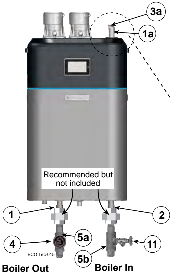
Figure 8 Install pipe fittings for relief valve and pressure/temperature gauge — DO NOT mount relief valve until AFTER hydrostatic testing (see legend below)
