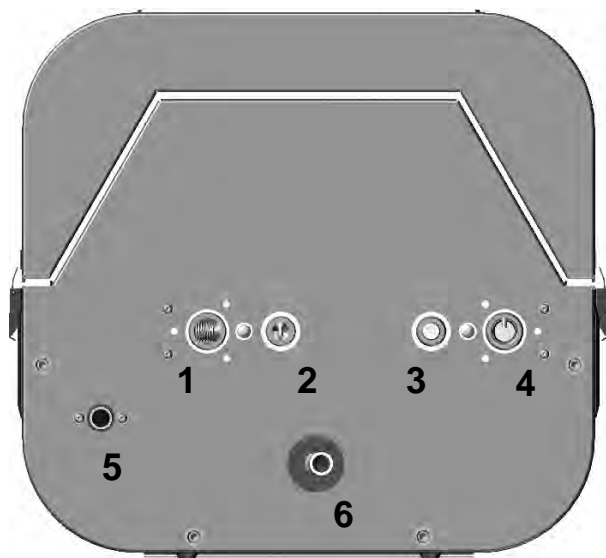
Figure 136 Boiler connections for cleaning domestic water circuit
