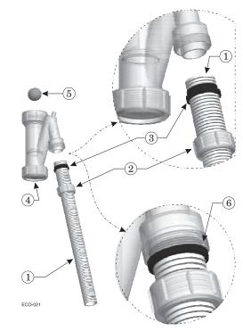
Figure 63 Condensate trap connection
