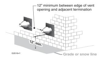
Figure 31 Installing and supporting the concentric sidewall vent assembly
