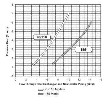
Estimated head loss of boiler loop piping and recommended circulators. Figure 51
