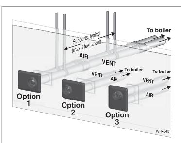
Vent/air pipes and vent/air can be oriented as option 1, 2, or 3. DO NOT mount with plate vertical and vent outlet down.
