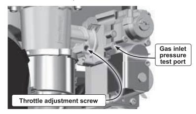
Adjust the throttle screw in small movements. Turning the **▲** CAUTION screw too far will cause the adjustment to reverse behavior.
