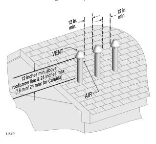
Figure 40 3" PVC concentric termination supports
