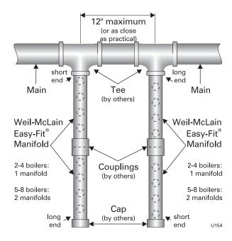
Figure 59 Double-sided EZ-Fit Header connection
