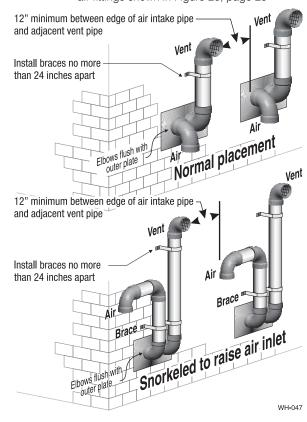
Figure 28 Sidewall termination assembly — using separate pipes
