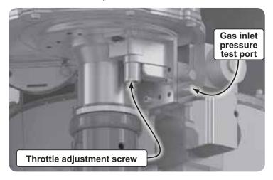
**ACAUTION** Adjust the throttle screw in small movements.
