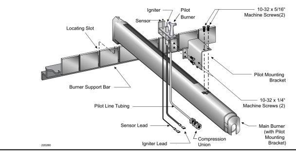
Figure 30 Main flame sense assembly
