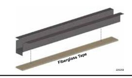
Figure 25 Back panel installation
