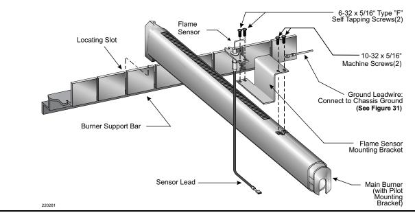
Figure 31 Main flame chassis ground
