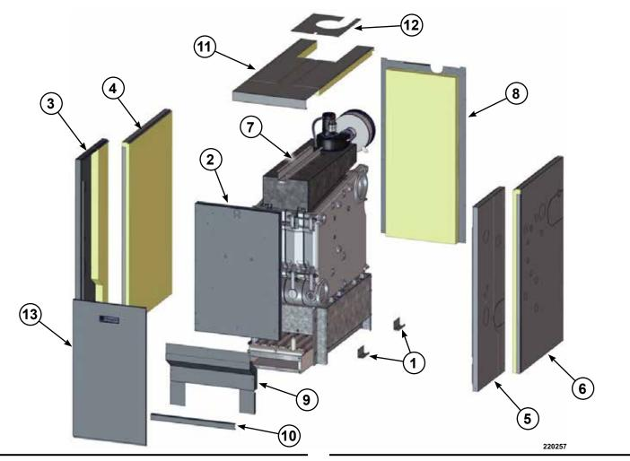
Figure 23 Front top interior panel installation
