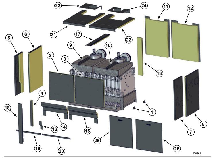
Figure 26 Recommended dual base jacket installation
