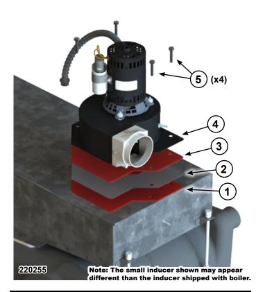
Figure 20 Inducer installation – steam boilers (except 4R)
