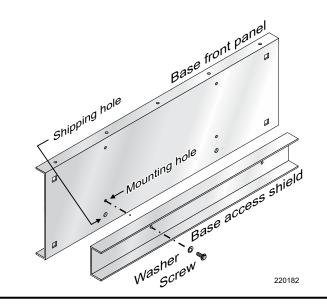
Figure 4 Shipping bracket removal
