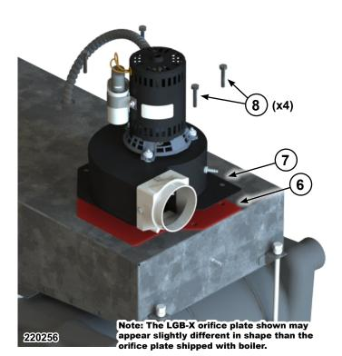
Figure 19 Inducer installation – water and 4R steam
