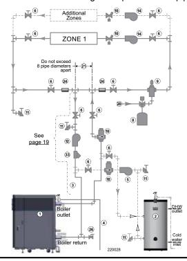
Figure 18 Radiant heating system with optional DHW
