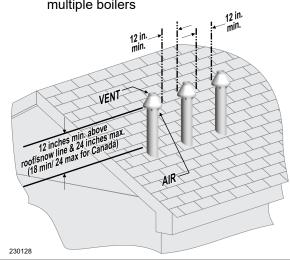
Figure 42 Concentric termination supports
