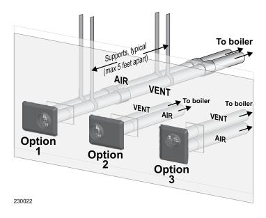
Figure 48 Adjacent terminations, vent and air plates – clearance from air inlet to exhaust
