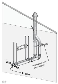
3. The air inlet of a boiler is part of a direct vent connection. It is not classified as a forced air intake with regard to spacing from adjacent boiler vents.
