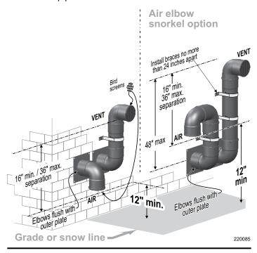
Figure 38 Multiple terminations, separate pipes – clearance from vent of one to air inlet of the next
