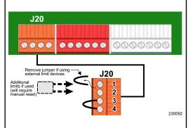
To cause AUTOMATIC reset: Connector J20 #3 & #4
