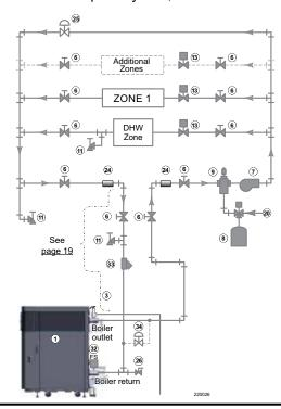
Figure 16 Variable primary flow, optional DHW piping
