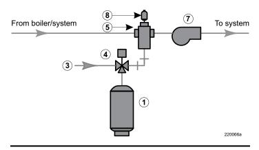
Figure 12 Expansion tank piping - closed-type tank
