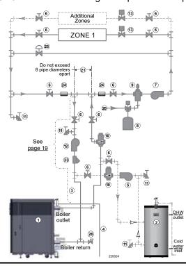
Figure 14 Zone valve zoning alternate with DHW piping
