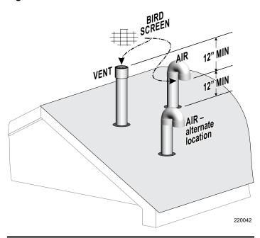
Figure 33 Vertical vent & air piping - termination location for multiple boilers
