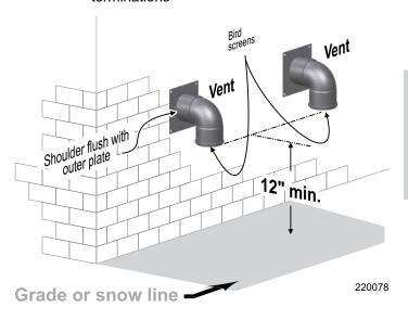
Figure 30 Sidewall termination assembly for direct exhaust installations
