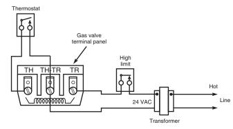
Figure 4. Wiring for 36C03/36C13 (24 Volt)
