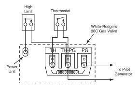
Figure 3. Wiring for 36C03U/36C13U/36D34U (.750 Volt)
