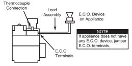
Figure 5. Wiring for Energy Cut-Off (E.C.O.) connection
