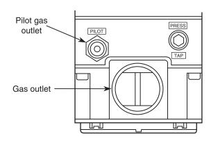
Figure 2. Gas valve side view
