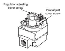
Figure 8. Pressure regulator adjustment
