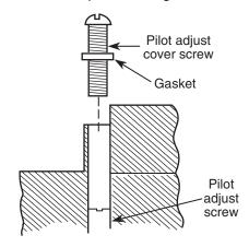
Figure 7. Pilot gas adjustment
