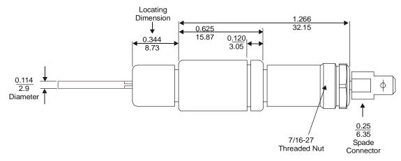
Figure 3: Y75A Dimensions, in. (mm)
