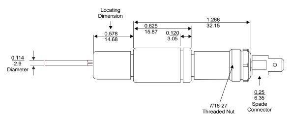
Figure 4: Y75B Dimensions, in. (mm)
