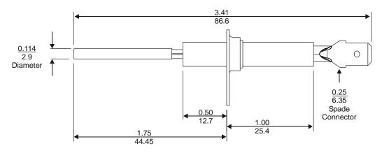
Figure 6: Y75MK Dimensions, in. (mm)
