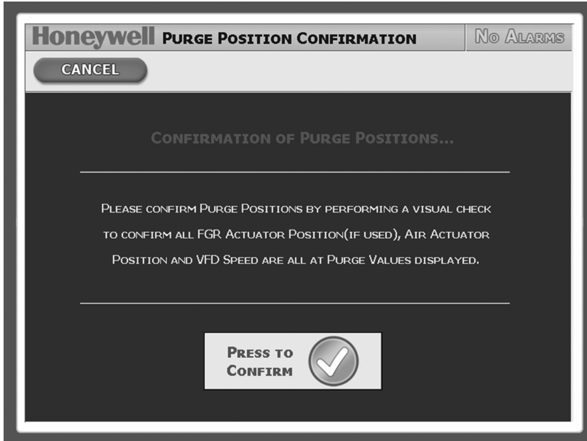
Fig. 33. Commissioning—purge confirmation screen.
