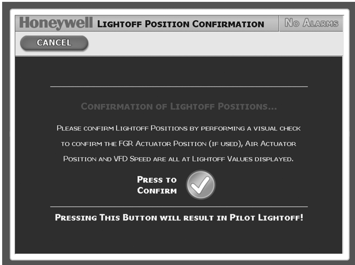
Fig. 36. Commissioning—lightoff position confirmation screen.
