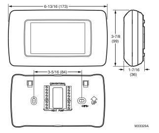
Fig. 3. Dimensions of THX9321 Prestige<sup>®</sup> 2.0 thermostat in in. (mm).
