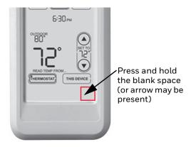
Fig. 46. Restarting the linking process.
