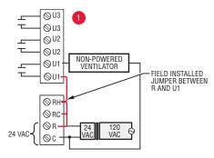
Fig. 348. Wiring a non-powered ventilator.
