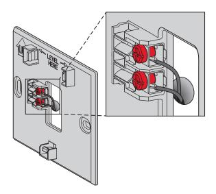
Fig. 20. Inserting wires in thermostat terminal screws (THX9421).
