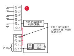
Fig. 347. Wiring a non-powered humidifier.
