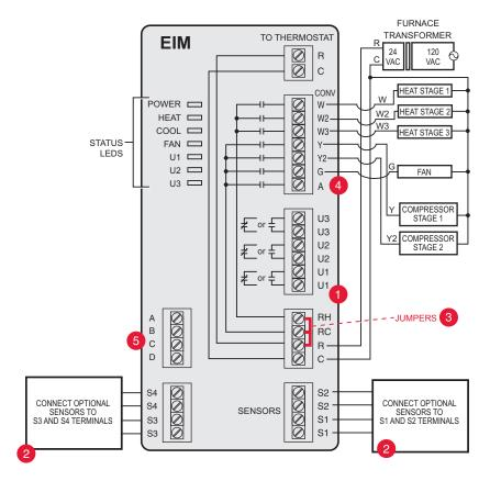
Fig. 324. EIM wiring guide - conventional systems.
