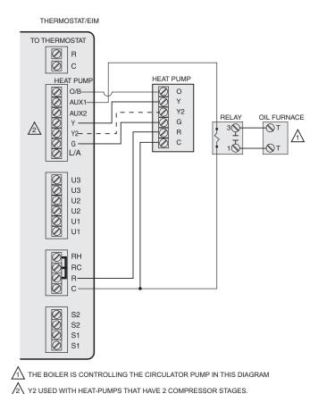
Fig. 336. Heat pump with oil forced air backup.
