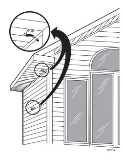
Fig. 69. Typical locations for C7089U1006 Outdoor Sensor.
