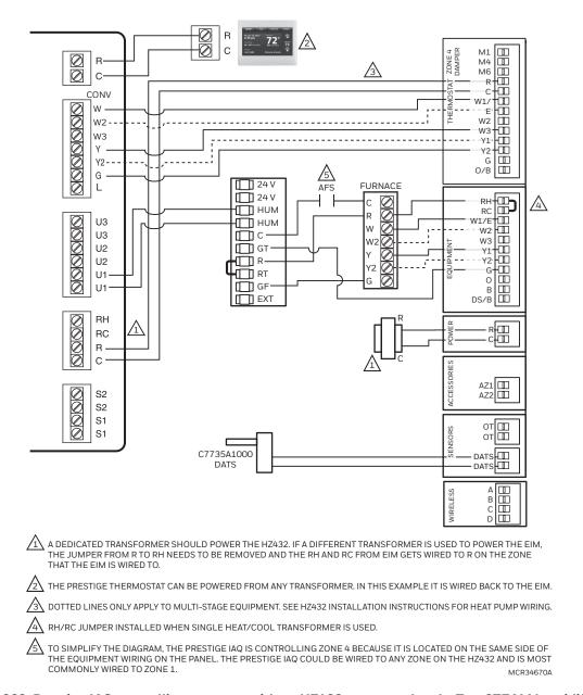
Fig. 362. Prestige IAQ controlling one zone with an HZ432 zone panel and a TrueSTEAM humidifier.
