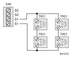
Fig. 359. Wiring 4 TR21 sensors.
