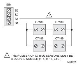
Fig. 357. Wiring 4 C7189U sensors.
