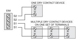
Fig. 187. Wiring dry contact devices.
