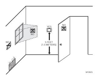
Fig. 16. Selecting thermostat location.
