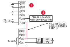
Fig. 349. Wiring a low speed fan for dehumidification.
