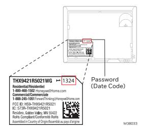
Fig. 6. Finding thermostat password.
