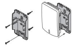
Fig. 70. Mounting Indoor Sensor.
