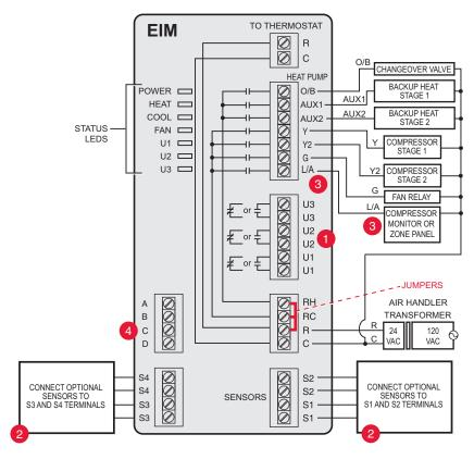
Fig. 325. EIM wiring guide — heat pump systems.
