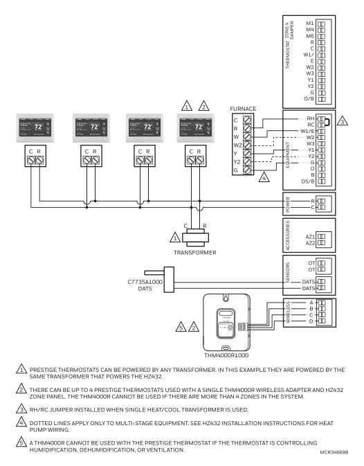
Fig. 361. Prestige IAQ thermostats with an HZ432 zone panel and no IAQ control.
