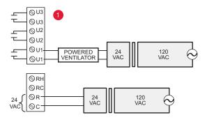
Fig. 345. Wiring a powered ventilator.
