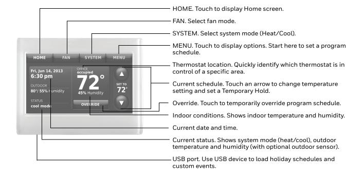
Fig. 75. Quick reference to commercial display.
