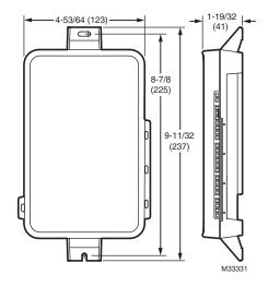
Fig. 5. Dimensions of Equipment Interface Module in in. (mm).
