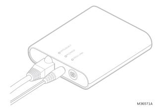
Fig. 47. RedLINK Internet Gateway connect button.
