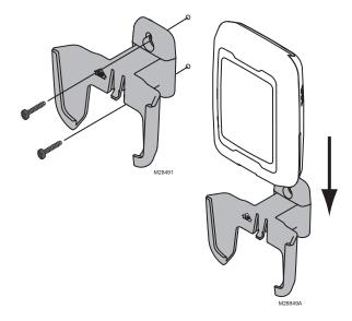
Fig. 68. Mounting Outdoor Sensor.
