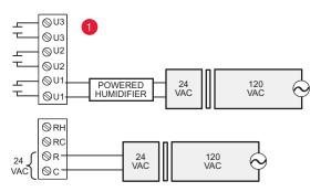
Fig. 344. Wiring a powered humidifier.
