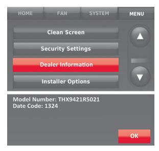
Fig. 55. Finding thermostat password.
