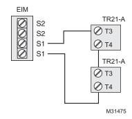
Fig. 360. Wiring 2 TR21-A sensors.
