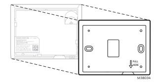
Fig. 17. Separate wallplate from thermostat (THX9421).
