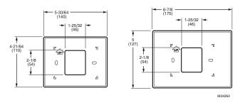
Fig. 2. Dimensions of THX9421 Prestige IAQ cover plates in in. (mm).
