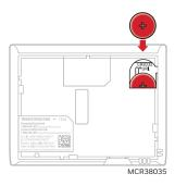
Fig. 19. Insert coin cell battery (THX9421)
