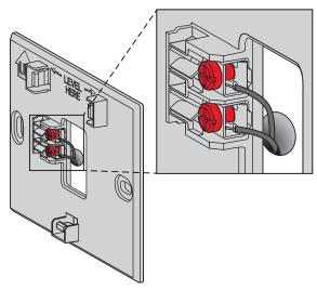
Fig. 322. Inserting wires in thermostat terminal block.
