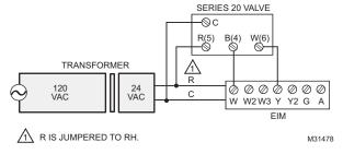
Fig. 334. Series 20 hot water heat.
